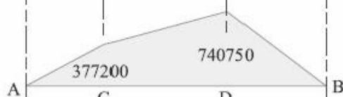
(f) Horizontal B.M. diagram.
